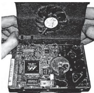
3.15-rasm. Vinchesterga sovitish qurilmasini o'rnatish.
