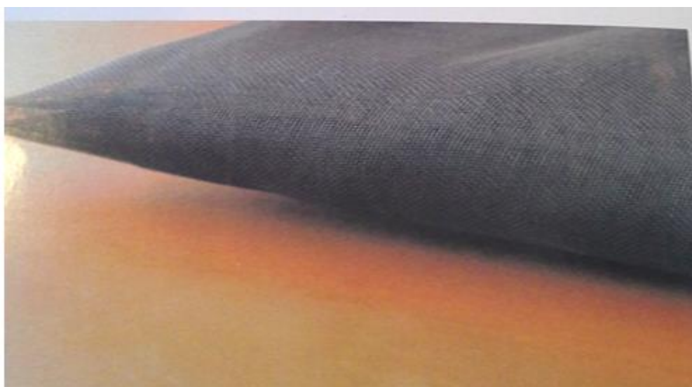
58-rasm. Titan nikeldan yasalgan membrana
